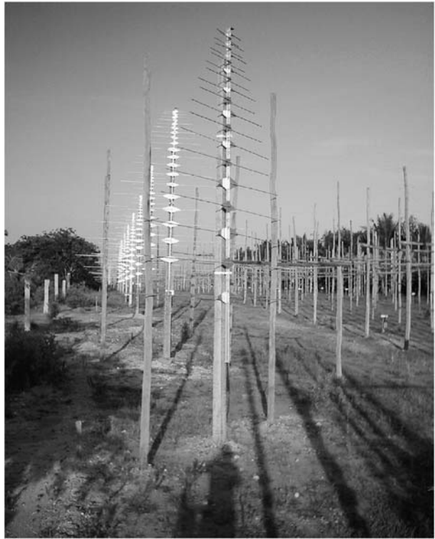
Figure 2 View of a section of the array. The orientation of the first LPD (near side) is 135^\circ and that of the second LPD is 0^\circ .
