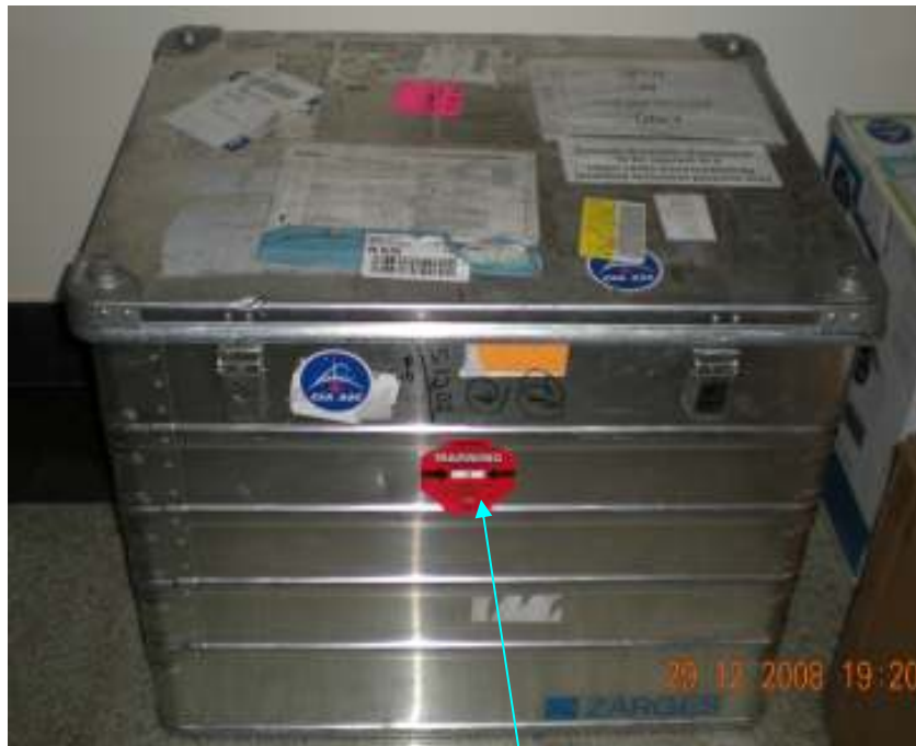
Figure 2. 1 HVU Box with RED Shock Watch Monitor
