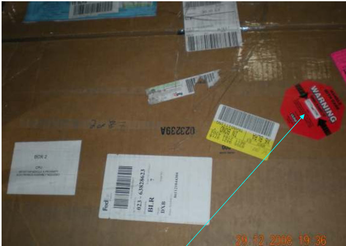
Figure 2. 2 CPU Box with RED Shock Watch Monitor
