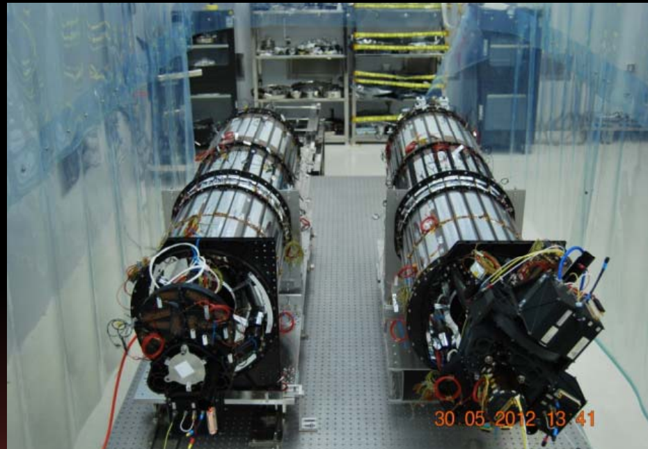
Purging with 99.999% Pure GN2 (UHP Grade)
