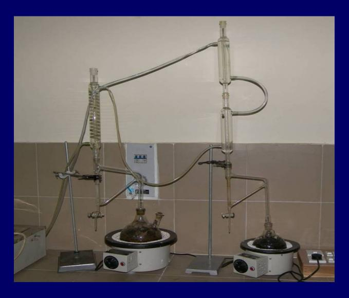
**Extraction of volatile essential oil fractions using Clevenger apparatus**
