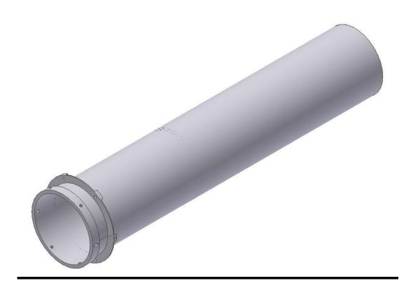
Fig 8: Primary Baffle Top Segment-PBTS.VIS (ref 2D drawing no IIA-UVIT-PL-PBTS.VIS)
