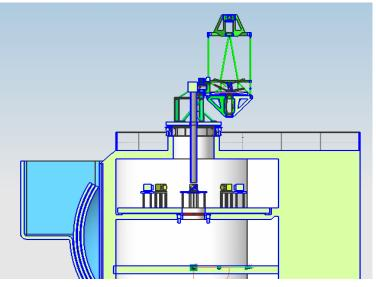
Figure 3: Cross section through telescope, instrument platform, and tower top
