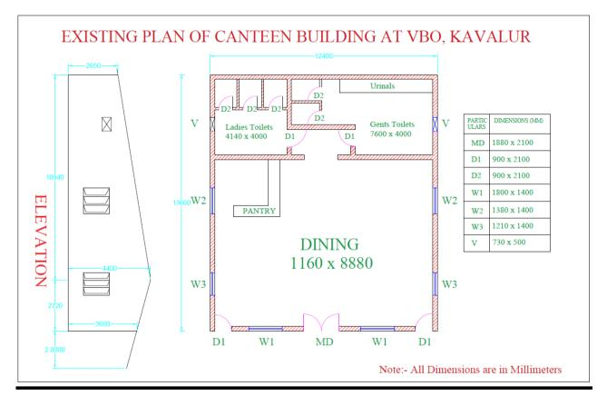
Note: The drawing is indicative may be referred for puff panel installation (roof) layout only
