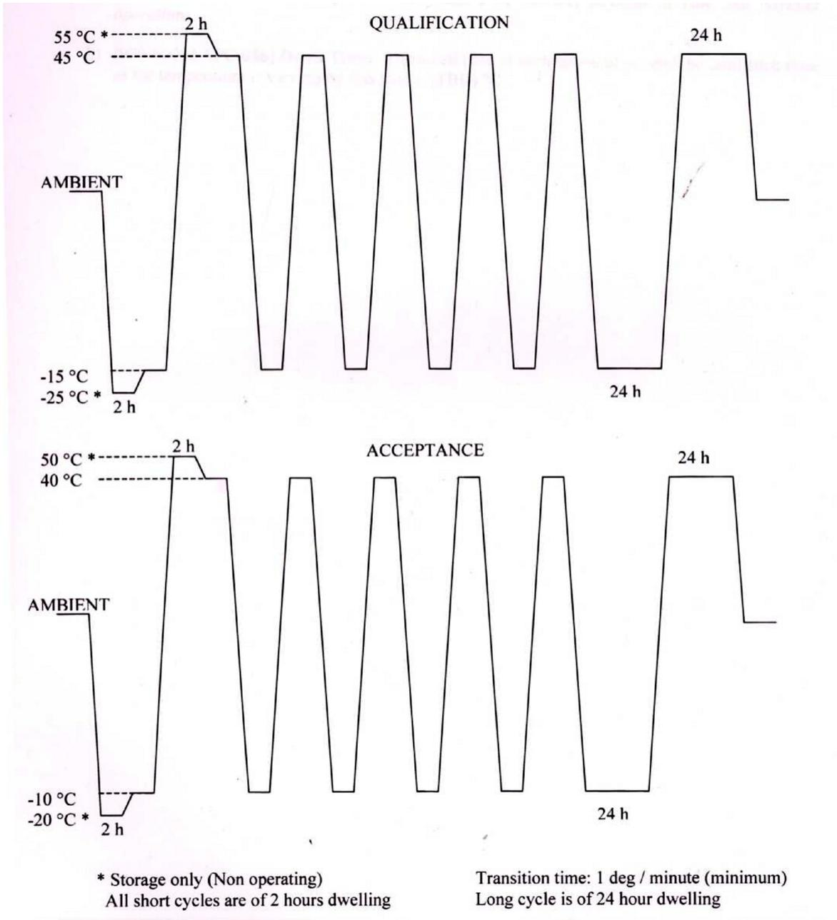
**Thermal Vacuum Test Profiles**
