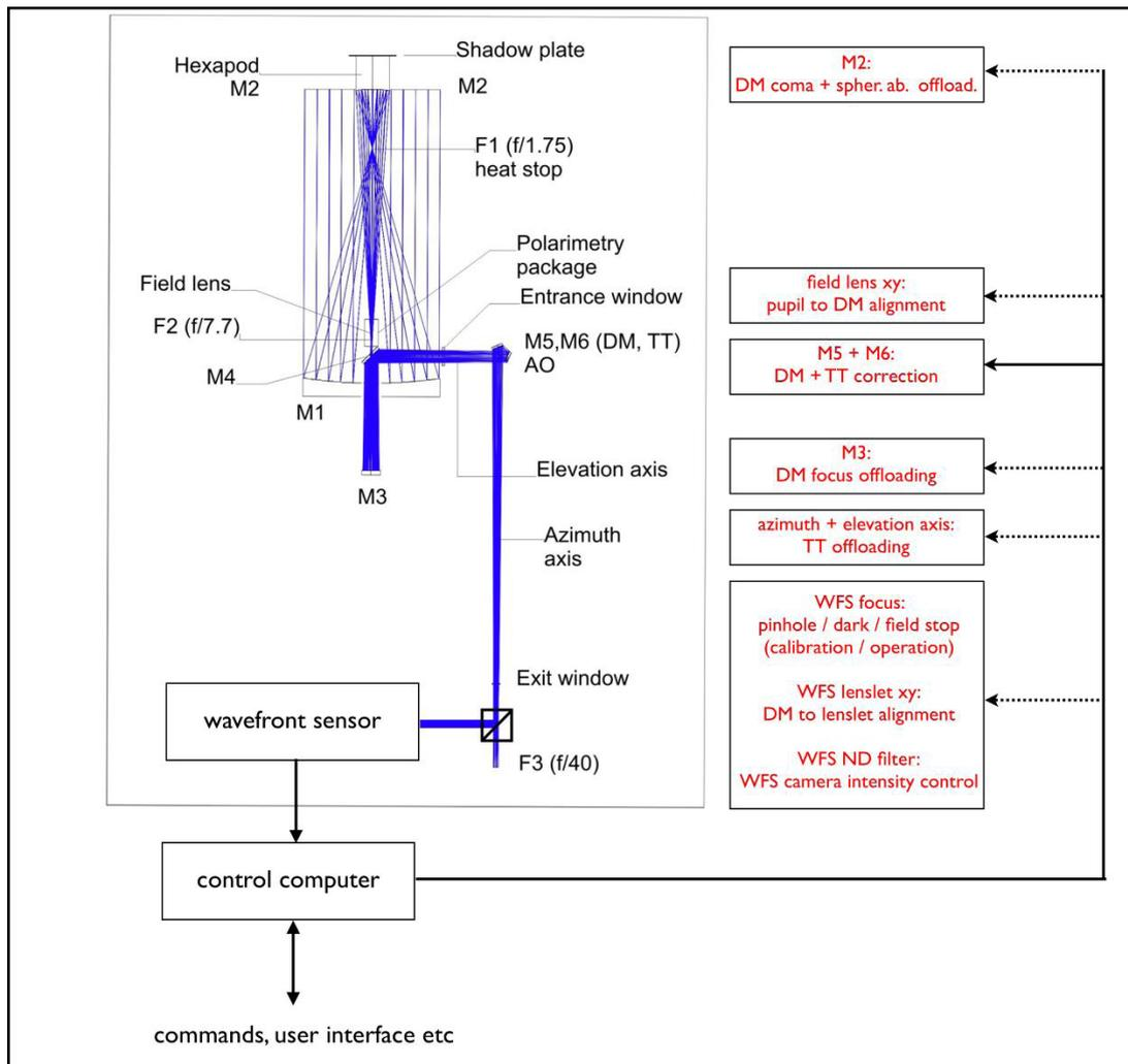
Figure 2: Adaptive and active optics control scheme
