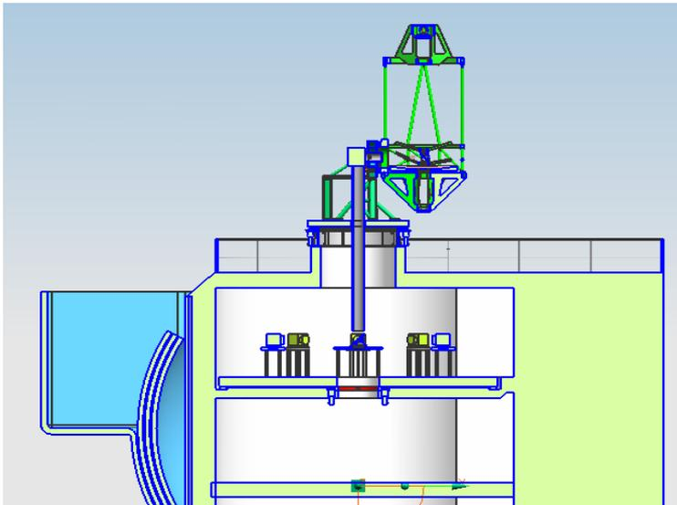
**Figure 3: Cross section through telescope, instrument platform, and tower top**
