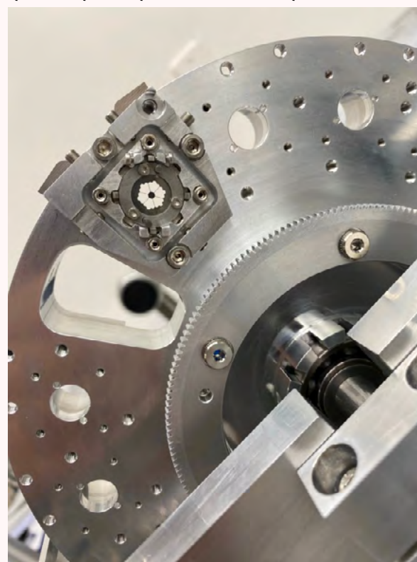
Picture 3: Left: Computer-aided design (CAD) of SCALES. Right: SCALES Lyot Stop mechanism (Credits: Author)
