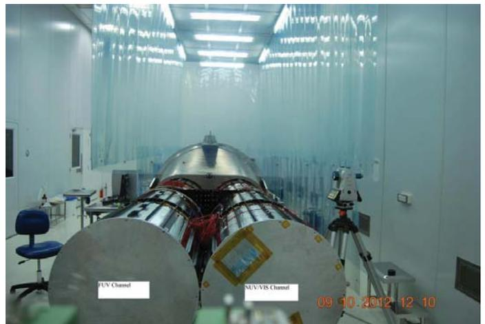
UVIT payload is to be launched on ASTROSAT and would make images in 28' field with a resolution < 2" in Far-UV (130-180 nm), Near-UV (200-300 nm), and Visible (320-550 nm). Testing and calibration of the two telescopes was completed. A photograph of the two telescopes shown above.
