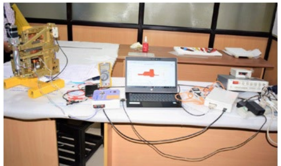
Figure 4: Actuators (P2e) undergoing Functionality testing at Southern Electronics, Bangalore, using ITCC's actuator functionality test equipment. (Image credit: ITCC/Prasanna Deshmukh)
