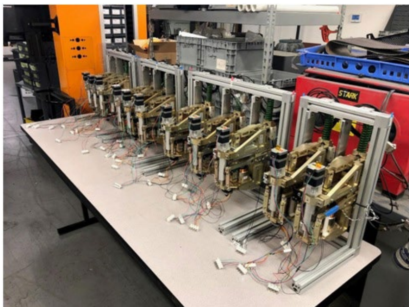
Figure 6: Actuators (P2e) installed on the Accelerated Life testing setup at The Pilot Group, California. (Image credit: TMT/TPG)
