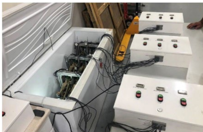
Figure 8: Actuators being life tested in cold conditions loaded into the freezer at The Pilot Group, California. Custom control boxes shown at right. (Image credit: TMT/TPG)
