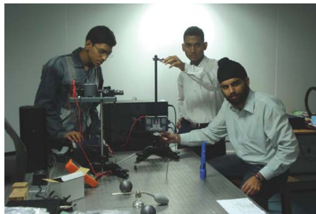
Students adjusting the torsion balance to measure the universal gravitational constant
