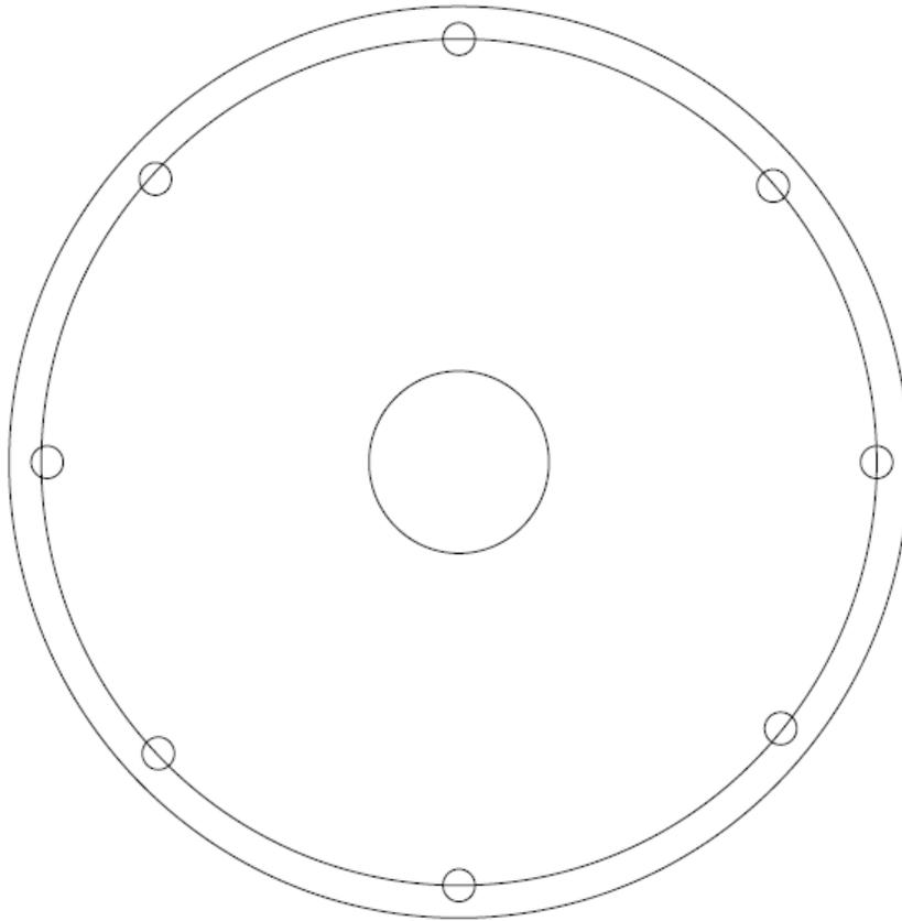
CCD FLANGE OD = 7 in [ 177.8 mm ]
