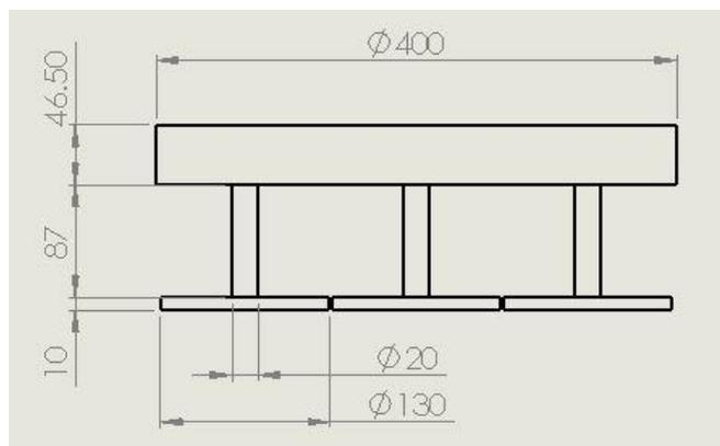
**Fig 3. Dimensions of Test Load**
