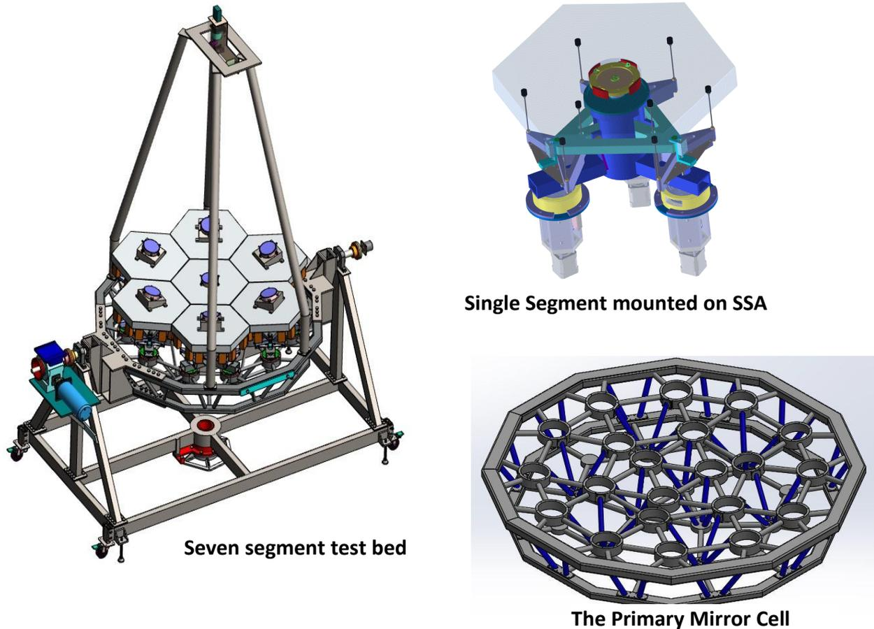
**Figure 1:** Mechanical model of the PSMT phase-I, which is a seven segment laboratory setup to test control of the segmented primary mirror.
