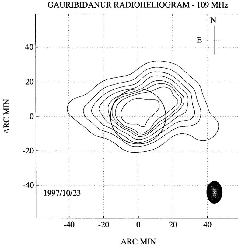
Figure 3. Radioheliogram obtained with the GRH at 109 MHz on 23 October 1997 at 06:30 UT. The contour levels are 79, 68, 57, 46, 35, 24, 13, 2% of  $1.02 \times 10^6$  K.
