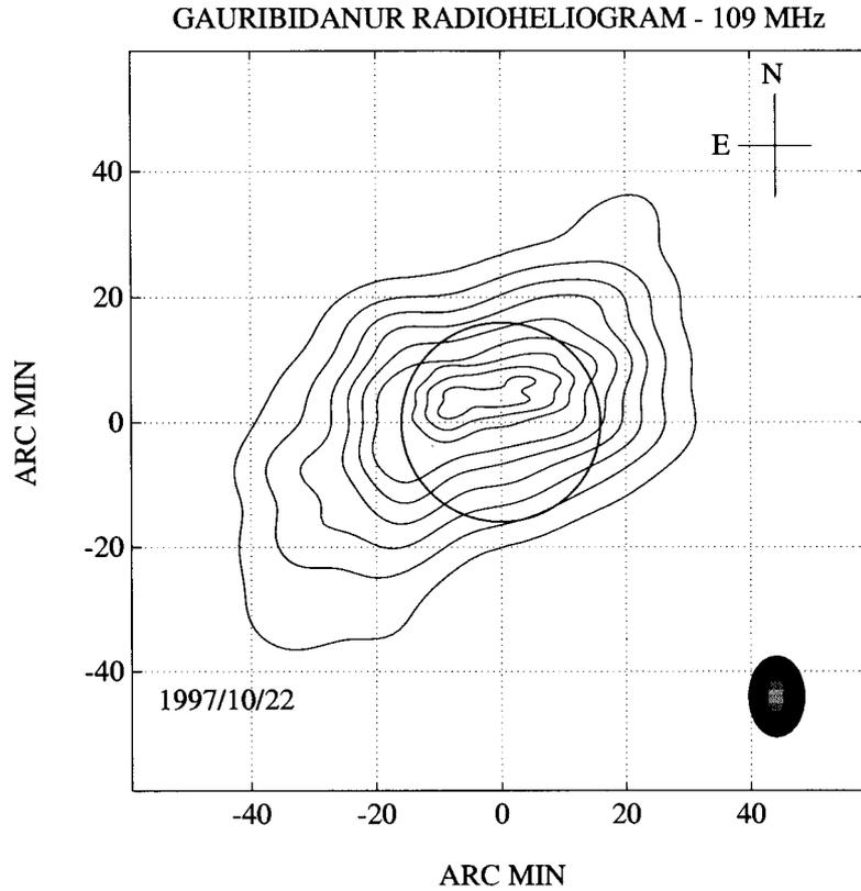
Figure 2. Radioheliogram obtained with the GRH at 109 MHz on 22 October 1997 at 06:30 UT. The contour levels are 82, 72, 62, 52, 42, 32, 22, 12, 2% of  $1.36 \times 10^6$  K. The open circle at the center is the solar limb and the filled circle at the bottom right is the beam of the instrument.
