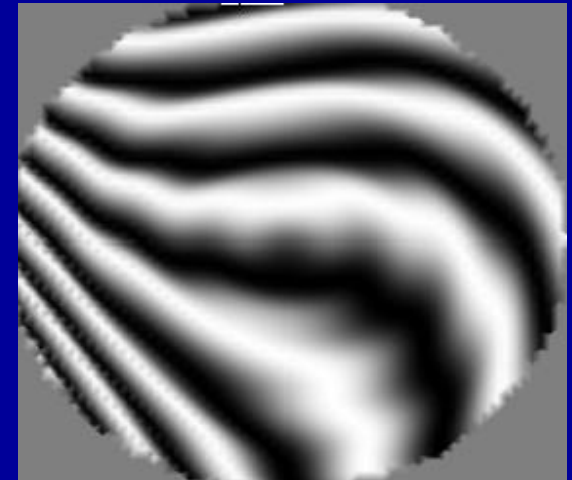
Errors due to turbulence
