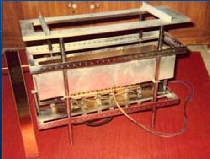
Gold coating Unit for SRBL Strip Mirrors
