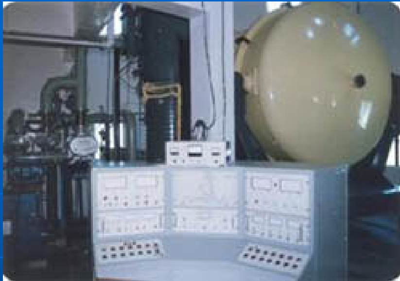
Gold coating Unit for SRBL Strip Mirrors
