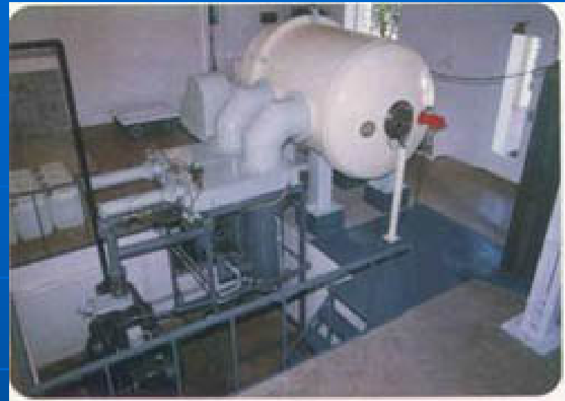
2.5 meter coating plant at IAO, Hanle
