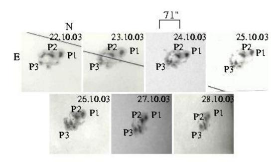
White light photoheliogram of the AR 10484 observed at Kodaikanal. The umbrae P1, P2 & P3 are taken for caluculating the changes in umbral orientations
