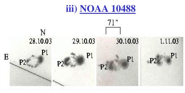
White light photoheliogram of the AR 10488 observed at Kodaikanal. The umbrae P1 & P2 are taken for calculating orientation changes
