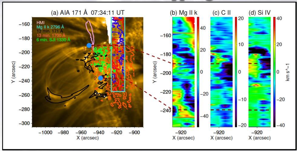
Pink contour: sunspot position seen in HMI Black contour: 6 min. oscillations in 171 Å Green contour: 6 min. oscillations in SJI 1330 Å Aguamarine Box
