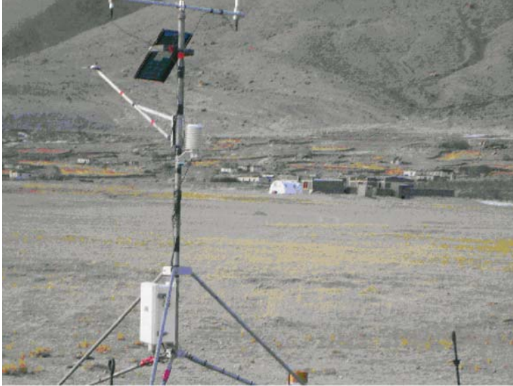
Figure 3. Weather station at Pangong to measure solar radiations, temperature, wind speed, etc.
