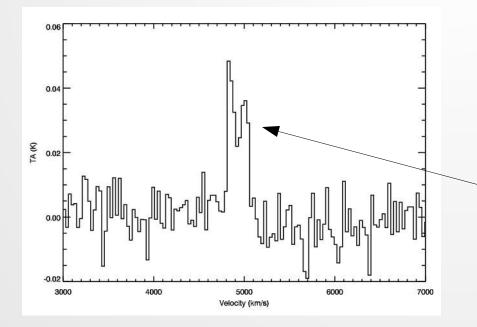
The figure shows the CO(1-0) emission line detected from the galaxy SBS1325 at 115GHz using the Nobeyama millimeter telescope (Das et al. 2015). Note the double horned profile shape indicating that the emissiion comes from gas in a rotating disk.
