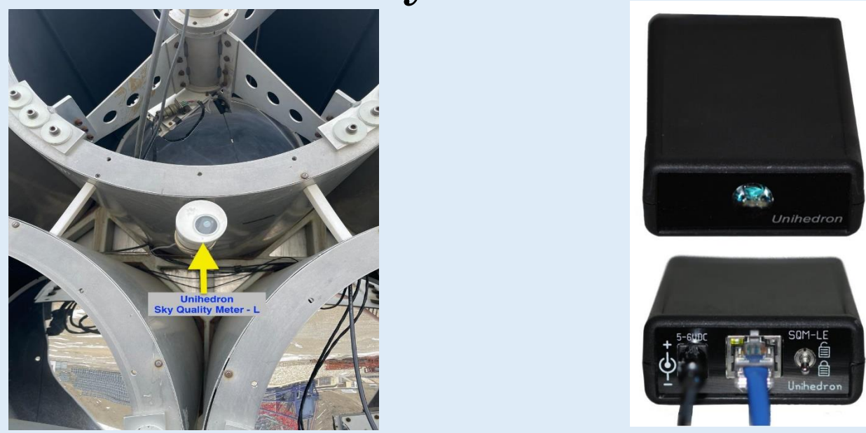
Unihedron Sky Quality Meter –LE is affixed to the central mirror of Telescope 7 and records data at 5 minute intervals.
